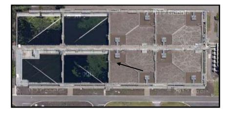
**Description:** Aeration Basin (Phase 2): Add step feed, anoxic selectors, and fine bubble diffusers to 4
