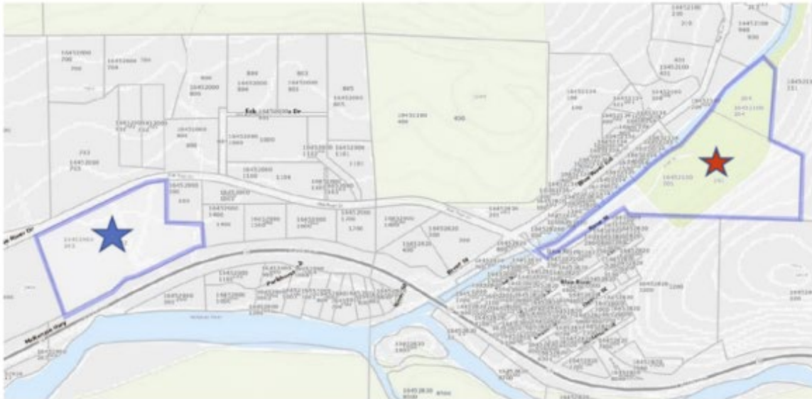
Figure 2. Identified potential wastewater drainfield sites. Blue River Park denoted by red star. Three Sisters Meadow site denoted by blue star.
